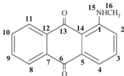
FIG. 1—The chemical structure of 1-(methylamino)anthraquinone depicts the stable three-fused ring aromatic system. Single chlorination occurs via a substitution reaction at the ortho- or para-positions relative to the methylamino substituent. The numbers in the figure label positions for unequivalent protons that will be referenced for  $^1\text{H}$  NMR resonances in Fig. 7.
