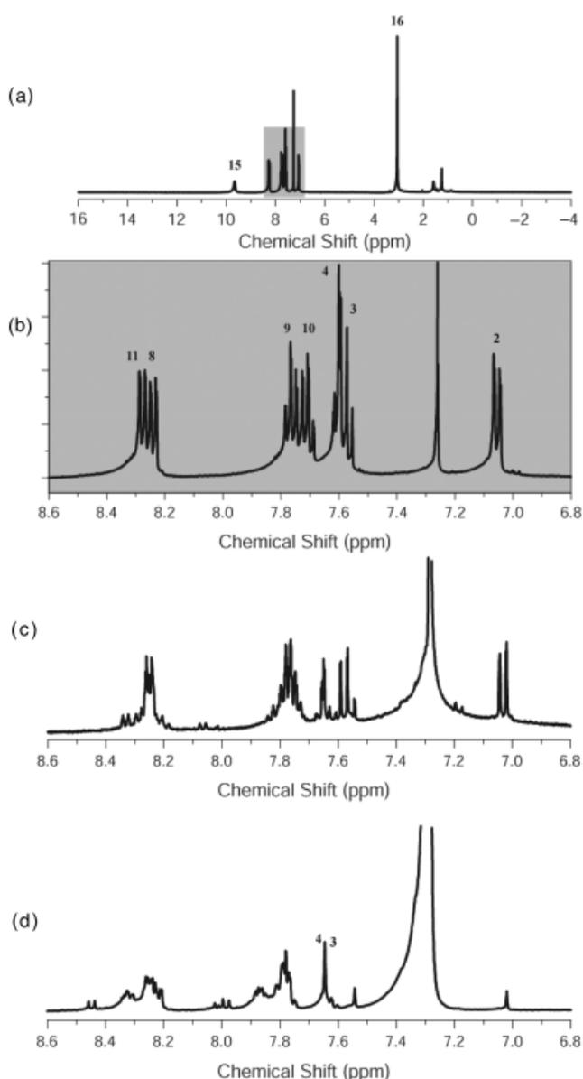
FIG. 7— $^1\text{H}$  NMR spectra for (a) 1-(methylamino)anthraquinone (MAAQ) and expanded  $^1\text{H}$  NMR spectra for (b) MAAQ, (c) para-chlorinated isomer, and (d) ortho-chlorinated isomer illustrate proton resonance changes after chlorine substitution.
