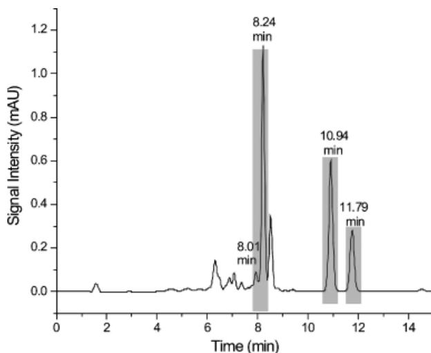
FIG. 5—Liquid chromatogram detected at 254 nm for the reaction mixture indicated a change in elution order between the two mono-chlorinated isomers. The shaded areas highlight the times used for individual fraction collection.
