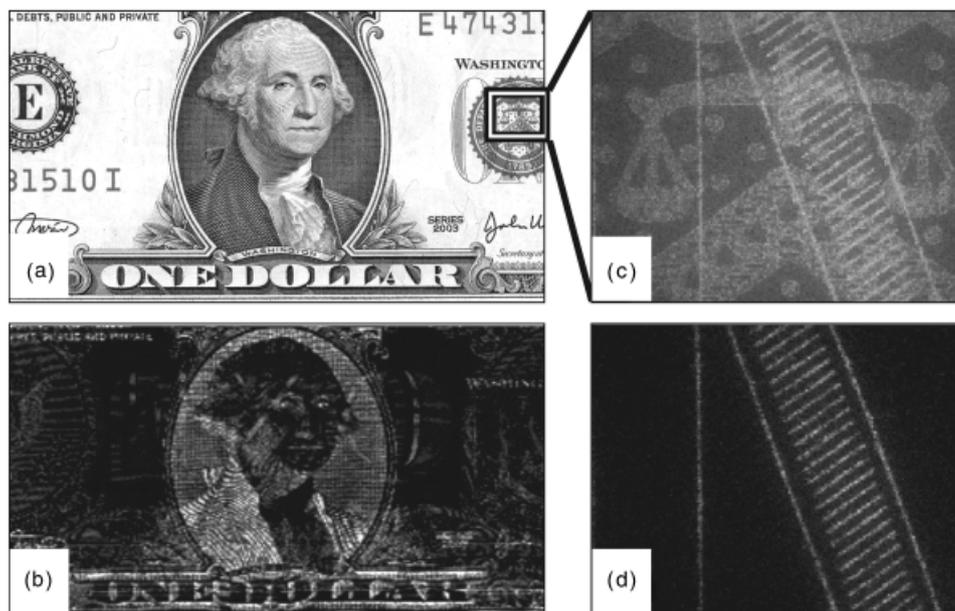
FIG. 8—Elemental iron maps of a dollar bill indicate that iron content correlates directly with black ink location. (a) Mosaic image of a dollar bill; (b) micro X-ray fluorescence elemental map of iron ( $K_{\alpha}$ ); (c) Scanning Electron Microscope (SEM) backscatter electron image of a dollar bill region where black ink overlaps the green ink of the treasury seal; (d) SEM elemental map of region (c) showing that iron is associated with black, but not green ink.
