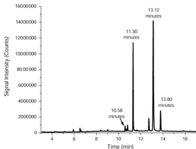
FIG. 3—Total ion count gas chromatogram for the mixture after catalyzed bleach reaction displays the unreacted 1-(methylamino)anthraquinone compound (10.58 min) and three reaction products: two mono-chlorinated isomers (11.30 and 13.12 min) and a di-chlorinated product (13.80 min).
