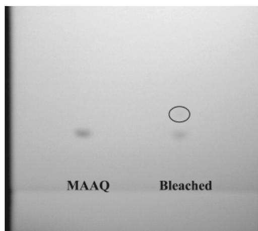
FIG. 2—Thin-layer chromatography plate was developed with two separate solutions spotted side by side. On the left is the 1-(methylamino)anthraquinone (MAAQ) standard at 1 mg/mL and on the right is the reaction mixture after bleaching. The circle indicates the presence of a faint pink band that represents chlorinated reaction products.
