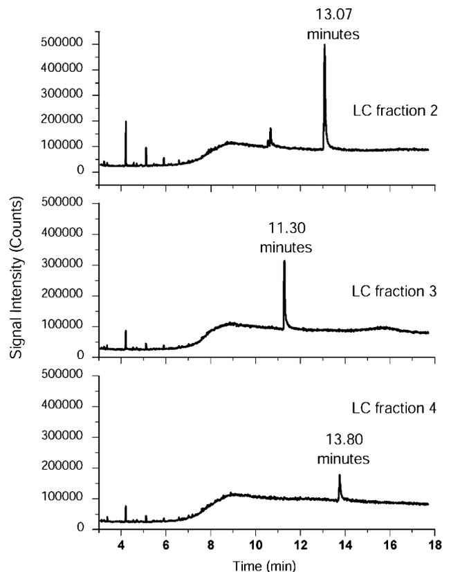
FIG. 6—Total ion gas chromatograms for each reaction product composed of 100 individual fractions collected in the liquid chromatography (LC) experiments. Mass spectra are not included but correspond to those contained in Fig. 4.
