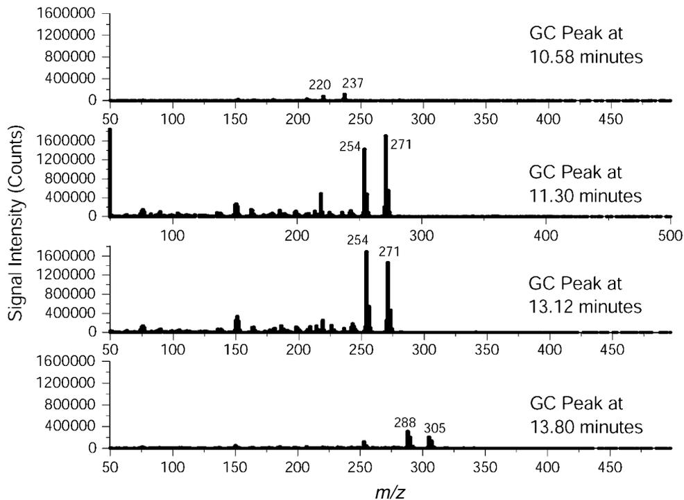
FIG. 4—Individual mass spectra at the maximum chromatographic peak heights indicate the presence of two mono-chlorinated isomeric compounds and one di-chlorinated compound.
